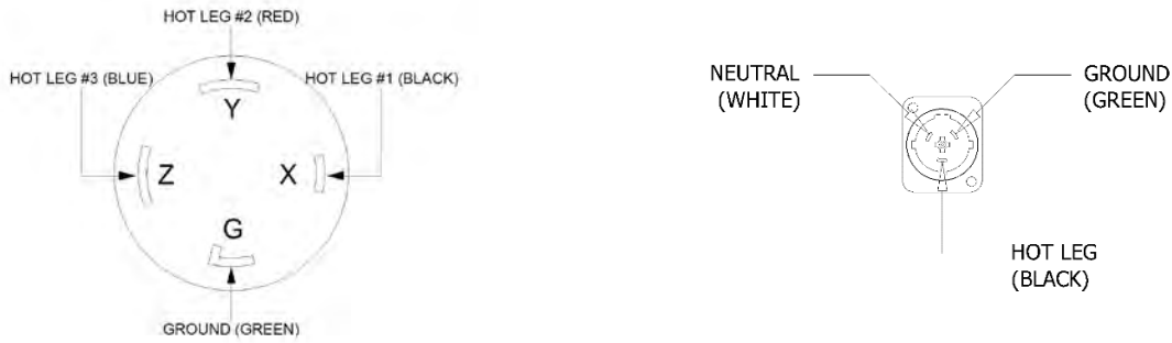
208VAC, 3 phase power connection
